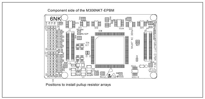
Figure 2.17 Positions of the pullup resistors
